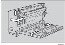
Open the rear cover by pushing the two knobs as shown in the illustration.
