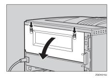
Remove the rear cover in the horizontal direction.
